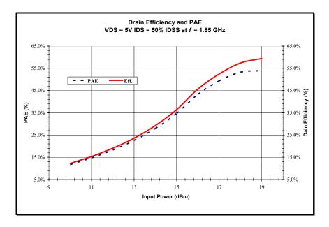
Typical power and efficiency is shown above. The devices were biased nominally at  $V_{DS} = 5V$ ,  $I_{DS} = 50\%$  of  $I_{DSS}$ , at a test frequency of 1.85 GHz. The test devices were tuned (input and output tuning) for maximum output power at 1dB gain compression.
